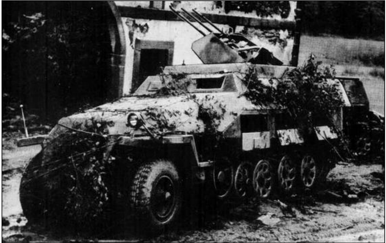
Hanomag Sd.Kfz 251/21 – German half-track with the three-barrelled 15 mm or 20 mm machine gun.
