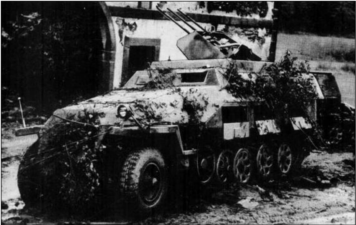
Hanomag Sd.Kfz 251/21 – German half-track with the three-barreled 15 mm or 20 mm machine gun.
